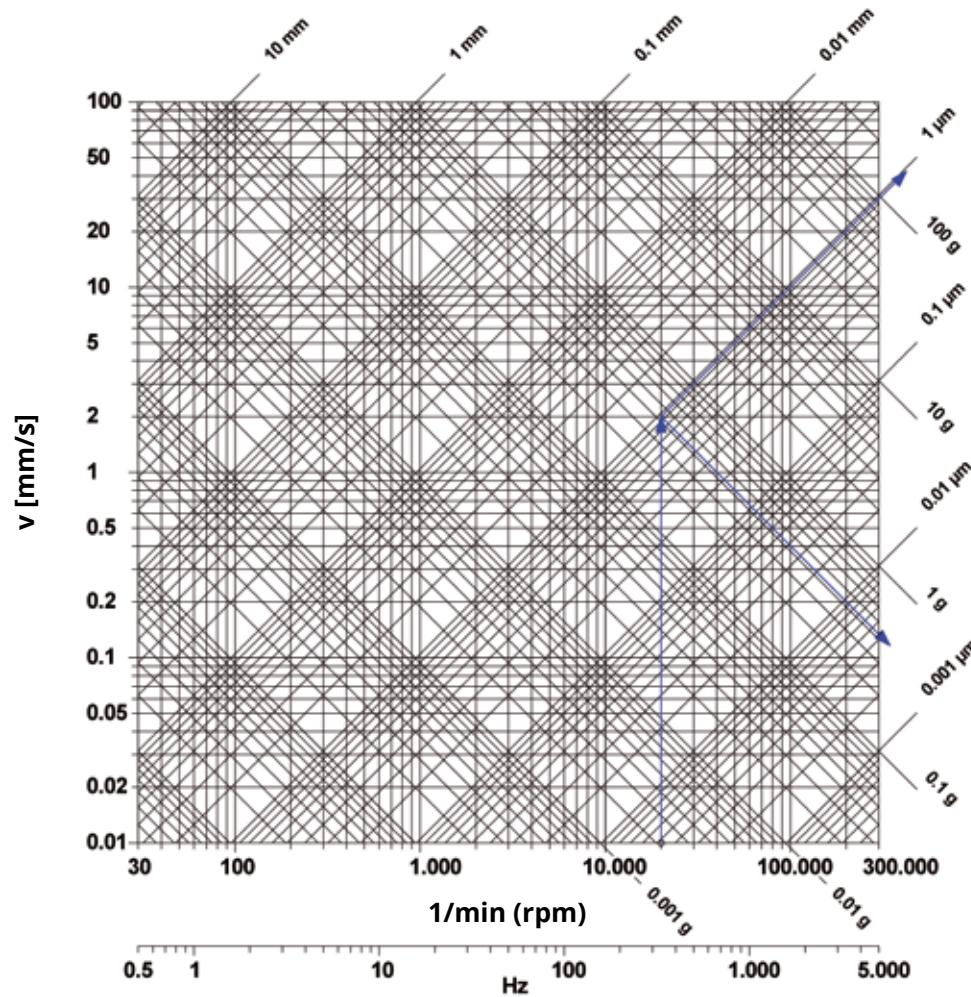
Example: 2 mm/s vibration velocity at 3.000 rpm or 50 Hz comply with appr.  $6.4 \mu\text{m}$  vibration displacement or  $0.031 \text{ g}$  vibration acceleration
